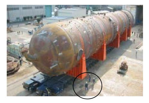
3 core 125 bbl/d F-T reactor pictured above a 4 core 175 bbl/d is available and a 6 core 250 bbl/d reactor soon. A - 4 core F-T reactor weighs approximately 23 tons
