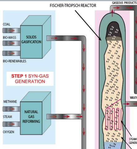
The Fischer-Tropsch Process (F-T) has three main processing steps shown here, all of which are commercially proven.
